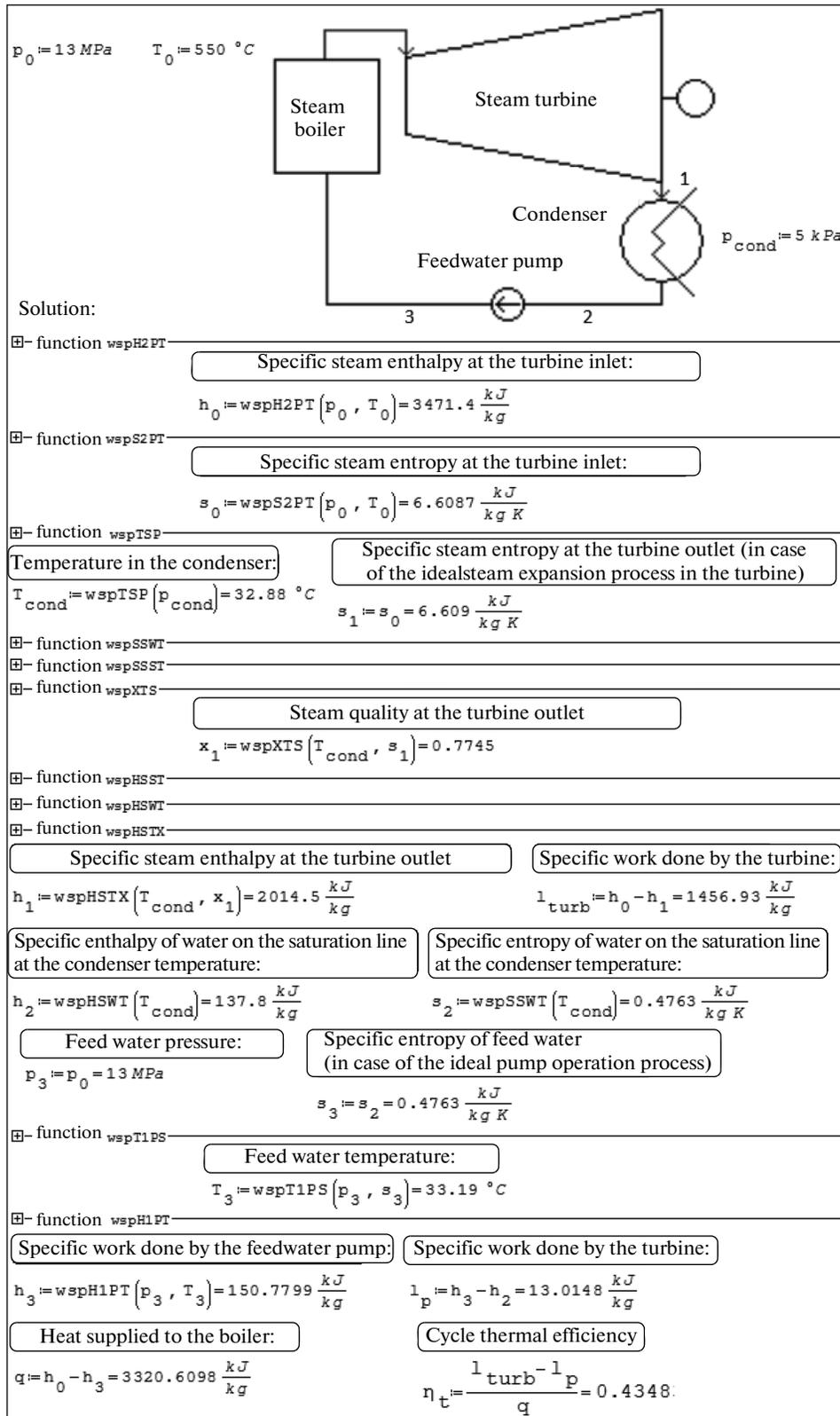
Fig. 6. Calculation of the thermal efficiency for the simplest steam-turbine cycle on superheated steam.
