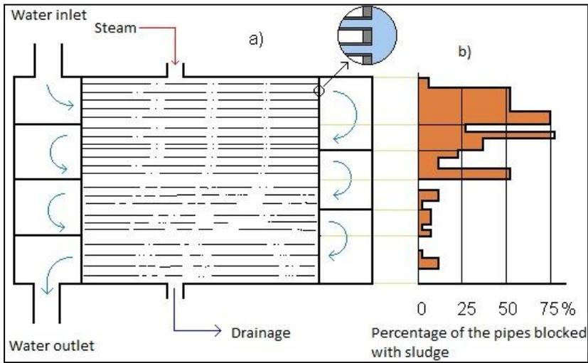
Figure 4. Blockage of the first heater by sludge
