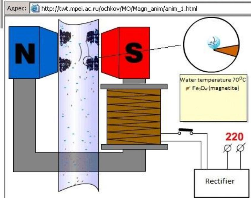
Figure 7. Scheme of the laboratory stand for studying effect of magnetic field on water solutions: 1 – thermostatic vessel containing initial water saturated with oxygen and nitrogen by bubble aeration, 2 – heat exchanger for water heating up to 70-80°C, 3, 6 - burette for measuring the volume of air evolved from water, 4 - dosing unit of ferromagnetic admixtures into the water, 5 – electromagnetic device, 7a, 7b – thermostats, 8 – vacuum pump, 9 – vessel for water collection
