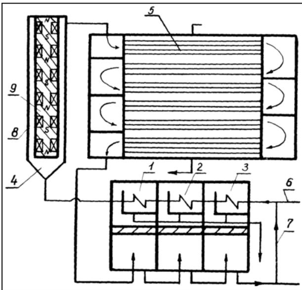
Figure 2. Scheme of three-stage adiabatic distilling system: 1-2 –distilled water collectors, 4 – magnetic apparatus, 5 – the first heater, 6 –source sea water, 7 – bypass of the hot sea water, 8 – gap of magnetic device, 9 – core of magnetic device.
