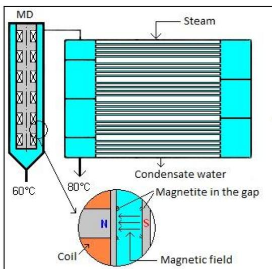
Figure 1. Connection of electromagnetic apparatus to the inlet of heat exchanger of water distilling system
