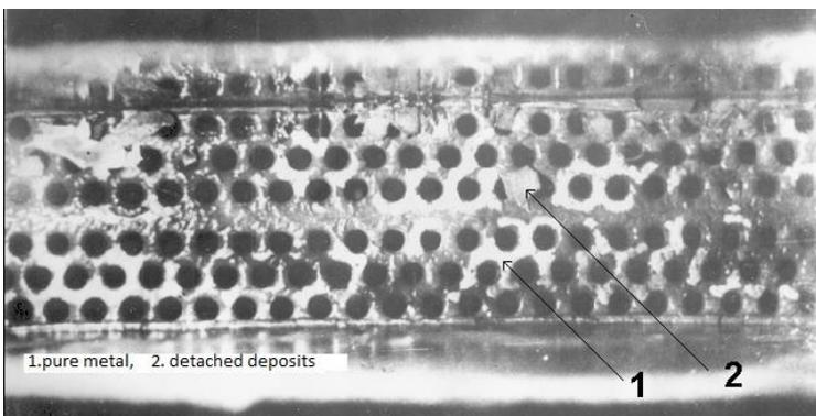
Figure 3. Picture of the tube plate of the first heater with scale
