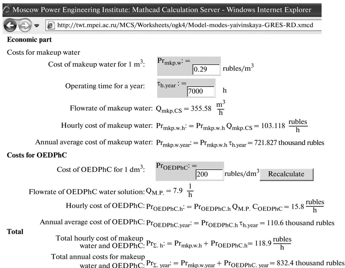
Fig. 3. Fragment of calculation by a mathematical model in the Mathcad environment (the economic part).
