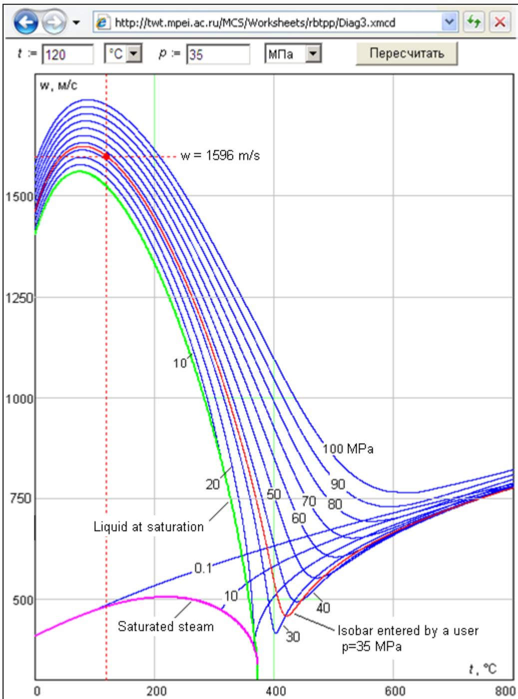
**Figure 3. Interactive network diagram of water and steam properties**
