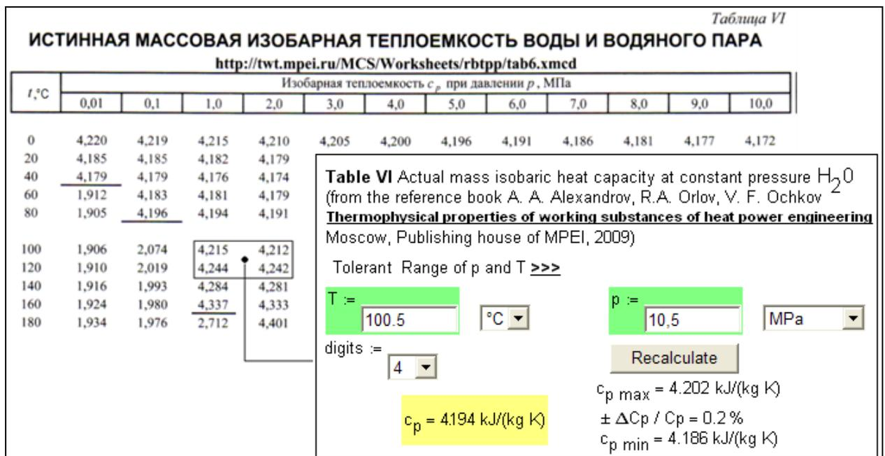
**Figure 2. «Paper» and on-line calculation of specific isobaric heat capacity of water and steam**
