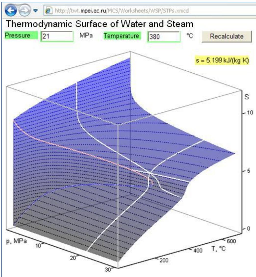
**Figure 4. Interactive network thermodynamic surface of water and steam**
