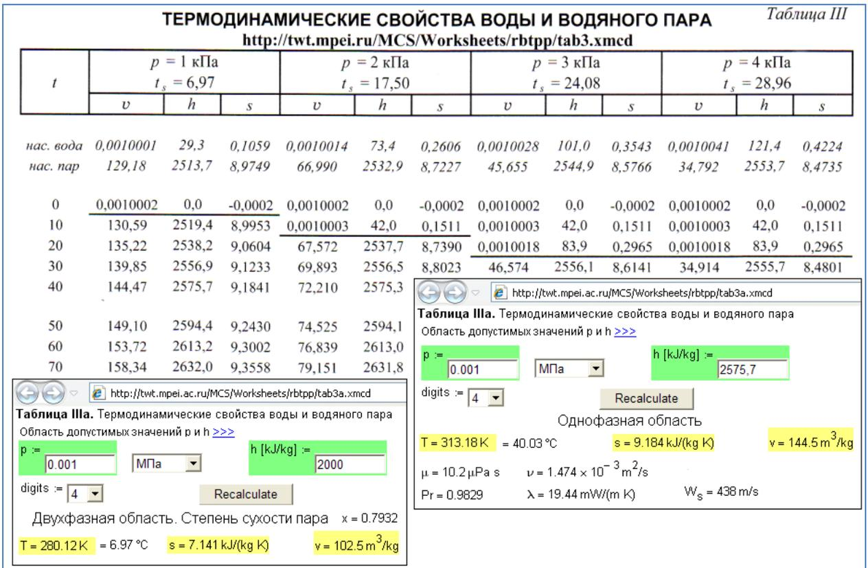
**Figure 5. «Paper» table and network calculation of water and steam properties**
